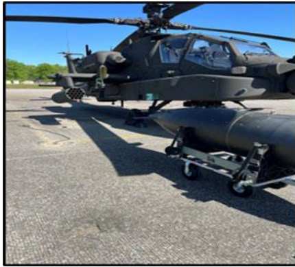
MIRC version 3 loaded with RCEF (front): AH-64 Apache helicopter wing loaded with Hellfire missile pod (rear).
