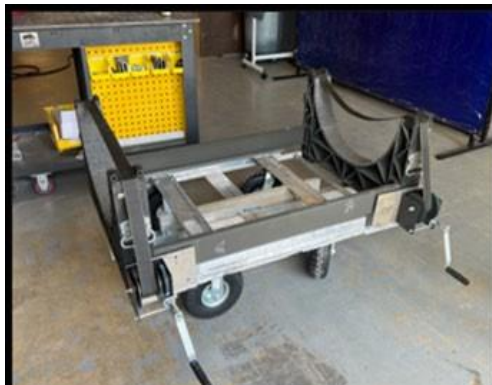
MIRC version 3 prototype with aluminum frame, lifting/lowering straps, and RCEF cradle.
