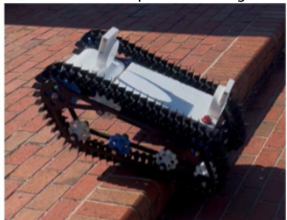
Fig 1. A CAPYBARA prototype ascends stairs
